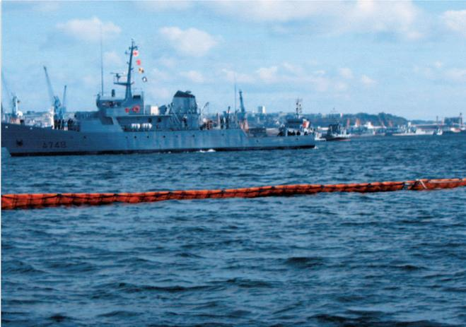
The containment boom « BARRACUDA » is intended to counteract the spread of hydrocarbon floating pollutions and is designed to be used on rivers and offshore.
